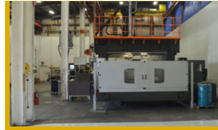
Napoleon Machinery's Toyoda LB63324M Bridge Mill in their 65,000 sq. ft. facility.
