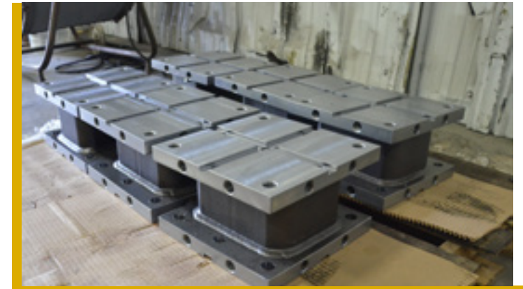
Custom designed riser blocks with the ability to be located on cross keys of Napoleon’s modular sub-tables. The shop fabricated, stress relieved and machined to specs the blocks in house.
